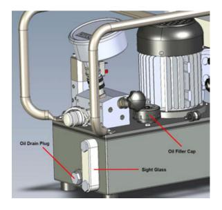
Run the pump in no load condition for 1 or 2 minutes maximum. Unplug the pump and remove the motor and pump assembly again. Now drain the flushing oil and re-clean the inside of the reservoir. (Make sure flushing fluid is also drained from pump assembly). Reassemble the pump and refill the reservoir with TorcUP hydraulic oil and reassemble the pump.
